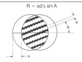
The wavefront radius, at the observation screen, is given by the following equation, with the wavelength, ' $\lambda$ , in the same units as S and d:
