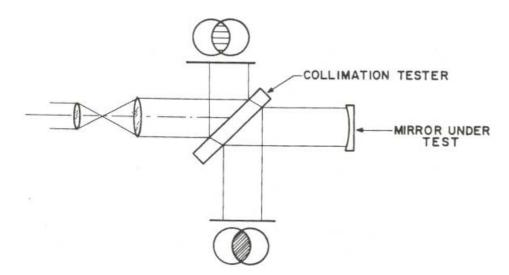
The wavefront radius at the mirror is calculated by adding or subtracting the mirror screen distance to the radius measured at the screen. The mirror radius is twice the wavefront radius. The collimation tester can also be used to measure optical material homogeneity as suggested by De Vany (5). It provides a simple method of obtaining single pass effects without the complications of a Mach-Zehnder interferometer.
